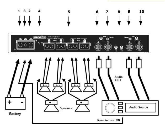
**1 – (BATT+)** POSITIVE power terminal block, connect it to the chassis oh the car or to the negative pole of battery (-).
